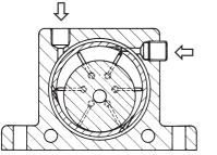
Housing made from extruded aluminium alloy
